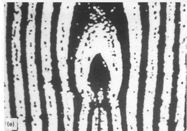
Figure 9 Moiré fringe patterns of the beam with a single-edge notch. (a) P = 15 \text{ N} , u ; (b) P = 20 \text{ N} , u ; (c) P = 24 \text{ N} , u ; (d) unloading, u ; (e) unloading, v .
